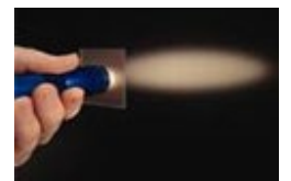
Filament Source 60° x 10° FWHM Elliptical
